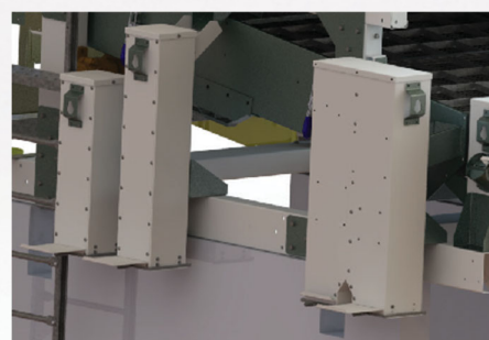
Laterally positioned bags remove various impurities processed through the filter boxes and suction chamber.
